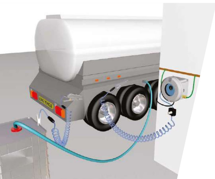
Example of grounded truck bonded to IBC
